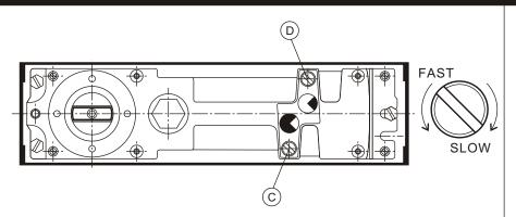
Closing speed The 7500 has two closing speeds which are independently adjustable.
